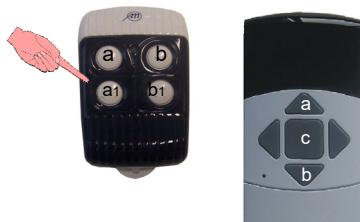
1. Press and release the learning key (LEARN) present on the card, selecting where to memorize the channel of the transmitter; relative red led turns on.
