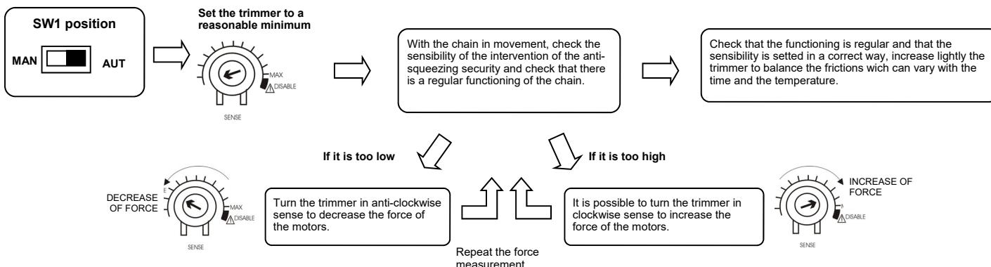
**Warning: With the trimmer in disabled position ( flashing light turned on), the anti-squeezing security is excluded.**
