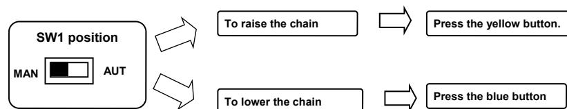
**WARNING: the reactivation of the automatic mode (AUT) implies the use of the reached position as totally closed position.**
