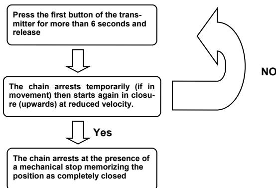
**Warning:** During the operation of resynchronization, the intervention of the anti-squeezing security is interpreted like identification of the closing position. To avoid the non-voluntary intervention the sense results remarkably reduced respect to the conditions of its normal functioning.
