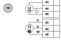
Connect the **230 Vac SINGLE PHASE** motor between the clamps 43 - 44 - 45.
