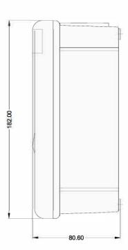
Overall dimensions: 140.50 x 182.00 x 80.60 mm Dimensions of the mounting holes: 114.00 x 156.00 mm
